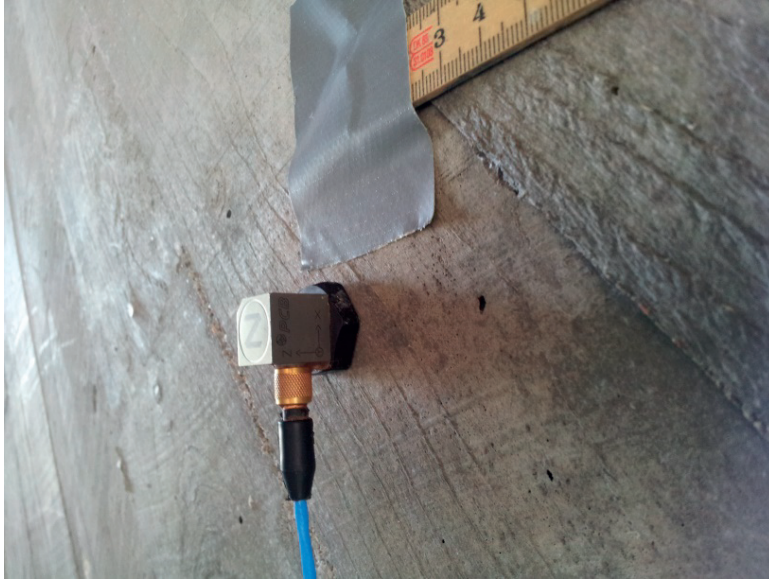
Figure 5.3: Three component accelerometer (PCB model 339A30).
