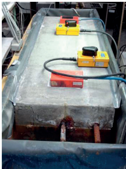
Figure 1.5: Example of mobile radar equipment used for measurement of concrete structure. Original figure presented by Lai et al. (2011).
